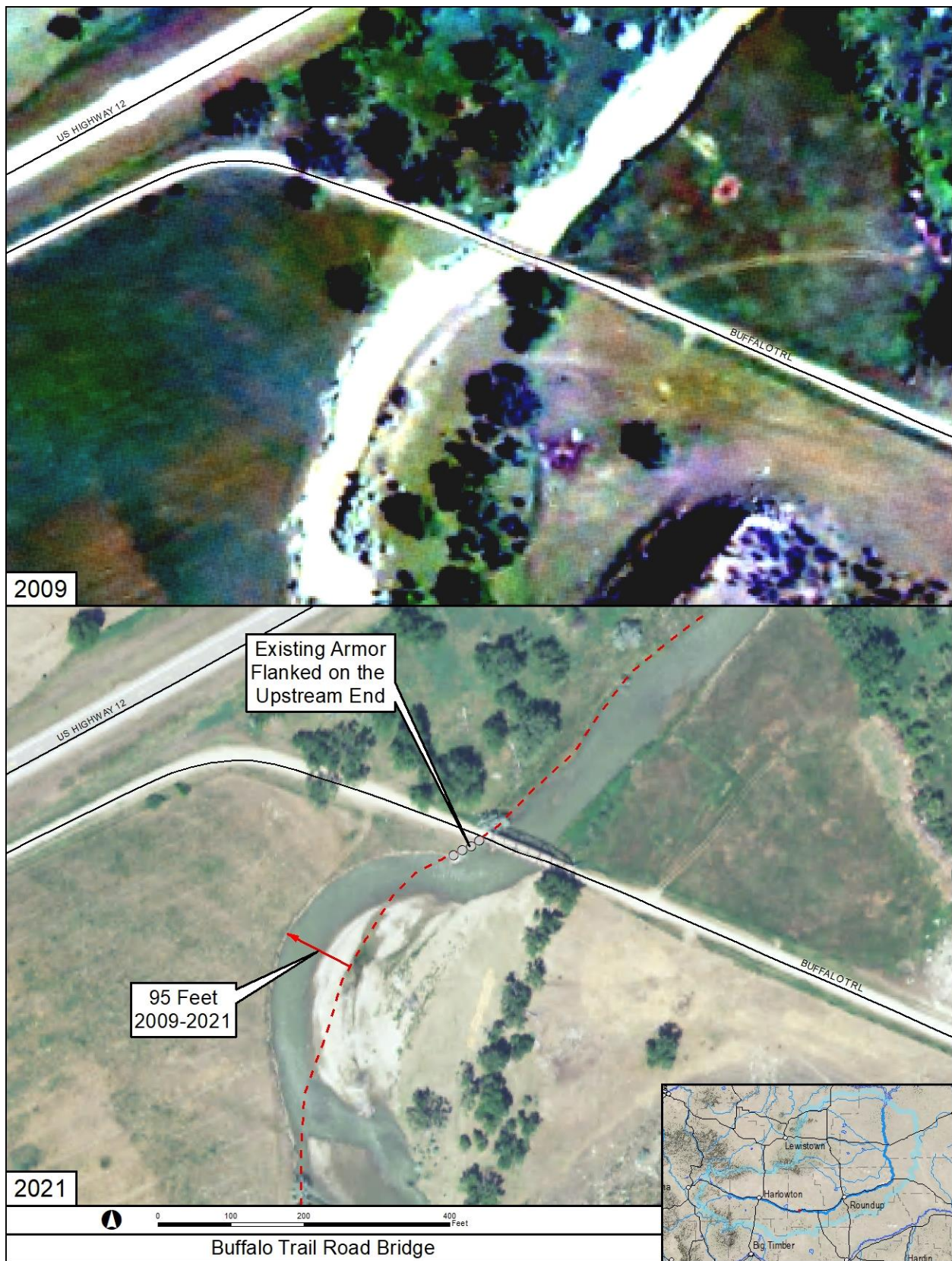
Figure 51. Aerial imagery from 2009 and 2021 showing left bank erosion just upstream of bridge.
