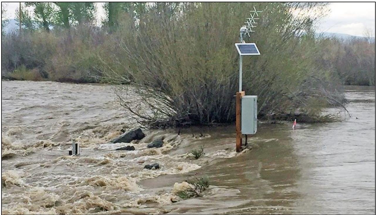
Figure 39. USGS stream gaging station on Big Wood River near Bellevue ID during a flood.
